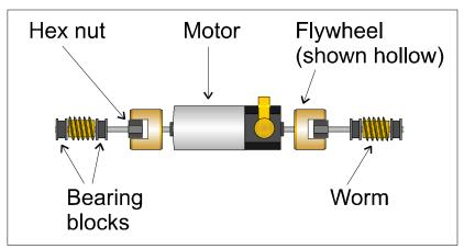
Here is a typical short axle split-frame mechanism drive train. There are essentially two parts: the motor with flywheels and the worm shaft assembly (one on each end).
