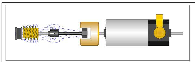
You do NOT want to remove the inner bearing blocks on locomotives that use a U-joint in the drive line. The u-joint would create an extra pivot point that would just allow the whole worm shaft assembly to flop around (as illustrated here). In this case, you want the inner bearing block because it is the u-joint itself that absorbs slight shaft misalignments.
