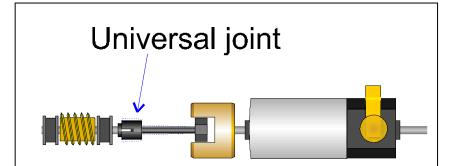
In longer locomotives, a universal joint can absorb a slight misalignment with no excess noise. This is the advantage of most 6-axle and longer 4-axle locomotives. Unfortunately, there just isn't enough room for a universal joint in shorter locomotives.
