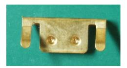
Recognize this? It is a bearing holder from an old Kato or Atlas locomotive. I needed a u-shaped piece, and this seemed like a good starting point.
