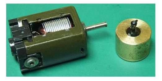
Getting all this off was not easy. If you can, you could try to pull that plastic piece off first. Then, it may be possible to hold the motor poles in one hand and twist the flywheel off. But don't do this with all your strength. I have had a situation where the flywheel held fast and the motor pole spun on the shaft- potentially damaging the motor! So go easy when trying to twist it off.
