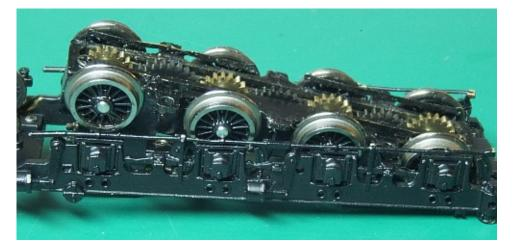
From the underside, the gearcase simply lifts out.
