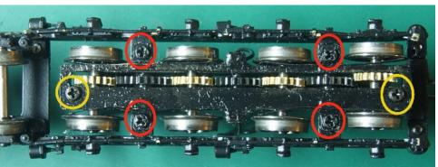
On the underside, there are 6 screws. The four screws indicated by red remove the gearbox from the sideframes.
