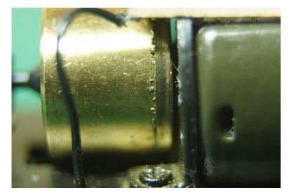
This flywheel was the worst, but the other had significant damage as well. Look at all the horrible metal particles that coming off of this. Not only does this cause dramatically high friction, but it also risks damaging the gears in the trucks.
