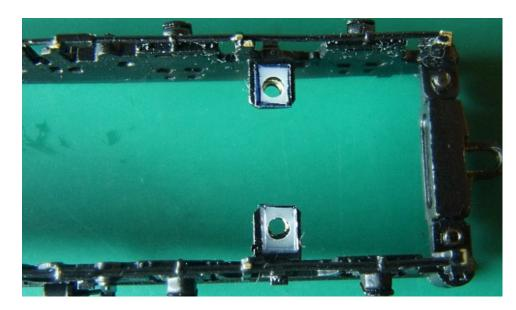
This is the UNDERSIDE of the sideframe assembly. Just lay the shim on each brace and re-insert the gearcase on top of it.
