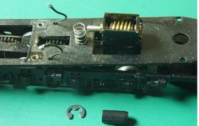
Remove the u-joint cup off the wormshaft. Pull the spring up and away.
