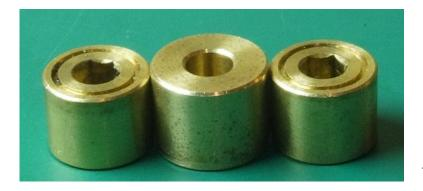
I was looking for a flywheel that was not only smaller, but also had a hex-nut interface that is typical of many high quality locos made by Atlas, Kato, and in some Life Like locos. These Life Like flywheels were perfect. They are a little smaller and have a hex nut hole into which I could insert a newer ujoint. I used a NWSL Puller to get the flywheels off.
