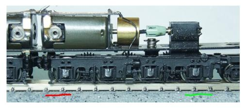
As stated on p. 4 of this document, it is clear from the wear spots that the underside of the sideframes sits too low and details scrape the track.
