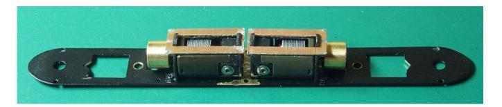
In the above shot, we have made new cut-outs for the geartowers, installed new flywheels and stabilized the motors. Time to move to the electrical system. It can be improved since those jumper wires are terrible.
