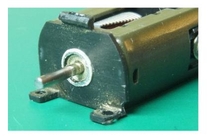
I installed the plastic motor mount over my taped bearing holder and it was just right- just a little snug. In fact, it went on better with a twisting in the same direction as the tape. This photo was taken for a test-fit, before I had cut the motor shaft.
