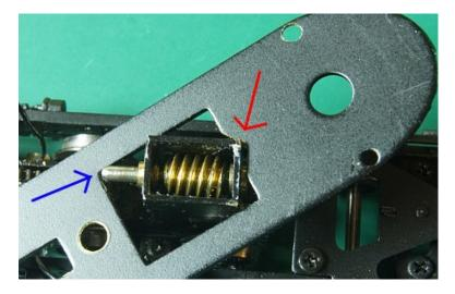
With the diamond point filed into the frame, the truck geartower now easily fits past the two tight spots.
