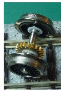
The wheelsets have some kind of fiberboard washers. They go on the OUTSIDE of the gearcase.
