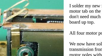
I solder my new flat "jumper" to the motor tab on the bottom (descretelydon't need much solder) and to the board up top.
