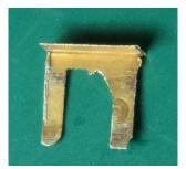
I cleaned up the burrs with minifiles. Here is the final product. I made two of these.
