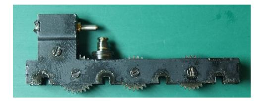
The gearbox itself is pretty simple. The gears are retained by screws.
