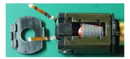
The rear cover has bumps that fit into the motor tabs to help lock them in place.
