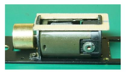
With flywheels in place, I mounted the motors back to the frame. I installed the back plastic motor mount on a motor and then installed the circuit board. Note that the boards have a skinny end and a fat end. The skinny end goes to the <u>back</u>, and the fat end goes toward the <u>flywheel</u>. This photo shows it **BACKWARDS** (it is easy to do).
