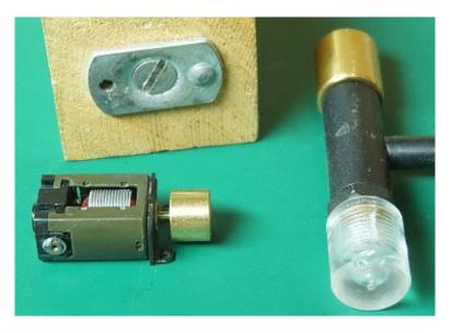
Installing the new flywheel was a little tricky since I had to hold the plastic motor mount in place. I placed the back of the motor on a hard metal surface and then gently tapped the flywheel down with a small hobby hammer with a plastic and brass head. I used the plastic head.
