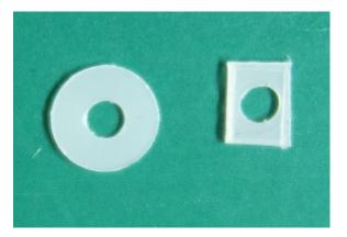
Raising the sideframe ended up being easy. I made shims out of Atlas thrust washers- 4 per truck.
