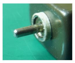
motor mount (there was not enough room for a NWSL Puller). Eventually I got the flywheel off without damaging the motor housing or shaft.
