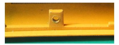
Since we are making design changes, let's solve a minor problem. This is the middle frame mount for the shell. When you remove the shell, or try and re-install it. These two tabs catch on the circuit boards.
