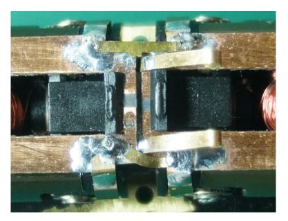
On test running the mechanism at this point, I found it stalled too often. I concluded that tying the motors together was essential so that both motors could draw from all available axles. And in fact, the stock model has a jumper wire between motors.
