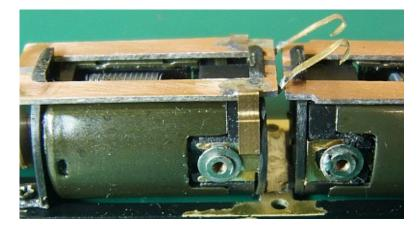
The tab catches at the middle of the loco where the two skinny sides of the circuit boards meet on top of the motors.
