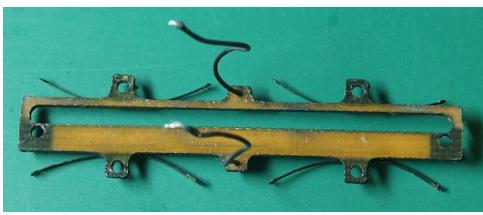
On the underside of the gearcase cover, you can clearly see that this is a perf board.
