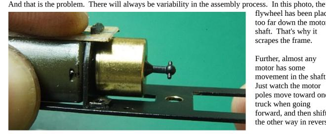
flywheel has been placed too far down the motor shaft. That's why it scrapes the frame.
