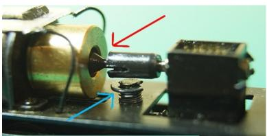
The trucks are drawbared together. So remove the screw between the trucks (red).
