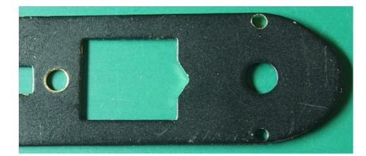
Now, frame is bare. Use a mini file to cut a triangle (sort of like a diamond point) out of outer edge of truck hole. Test truck fitting this hole by trying to get truck back on the frame. The triangle should allow the truck to fit into place with no trouble.
