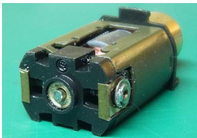
Notice the backside wraps around. When the back motor mount is installed, it will keep these new motor tabs pressed forward.
