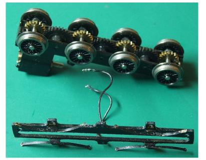
The bottom gearcase cover has the pickups soldered directly too it.
