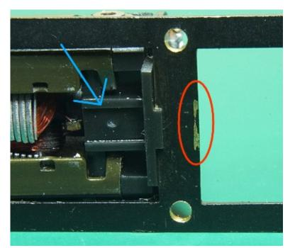
In fact, with the motor removed, the paint scraping (red) shows that this motor has indeed been vibrating back and forth.
