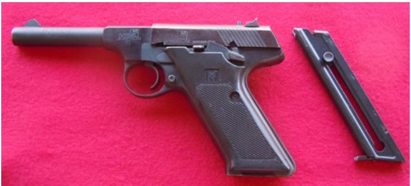
An Early version Iver Johnson Trailsman- note the button by the rear sight
